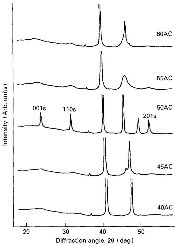
Figure 3 X-ray diffraction patterns of Au-Cu alloys aged at 170 °C for 500 h.
