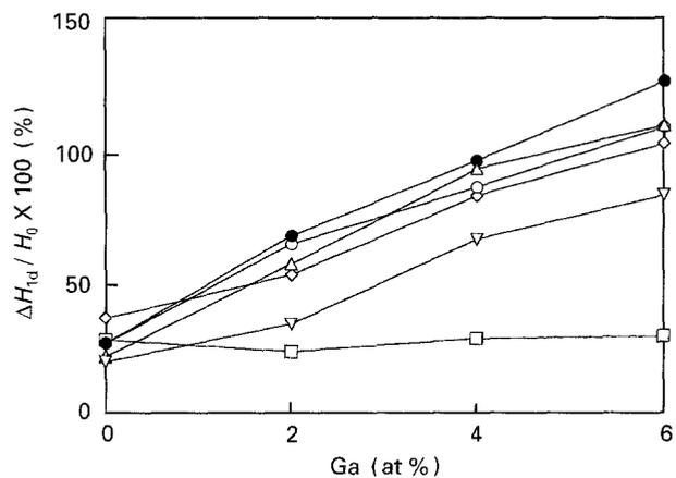
Figure 5 Relation between age-hardening rate and gallium content. Specimens were aged at 37 °C for 1 d: (□) 40AC-G, (○) 50AC-G, (●) 50AC-RepG, (Δ) 55AC-G, (▽) 60AC-G.
