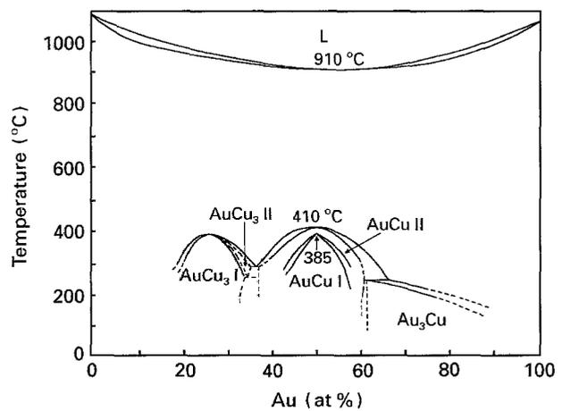
Figure 1 The Au–Cu equilibrium phase diagram redrawn from [4].
