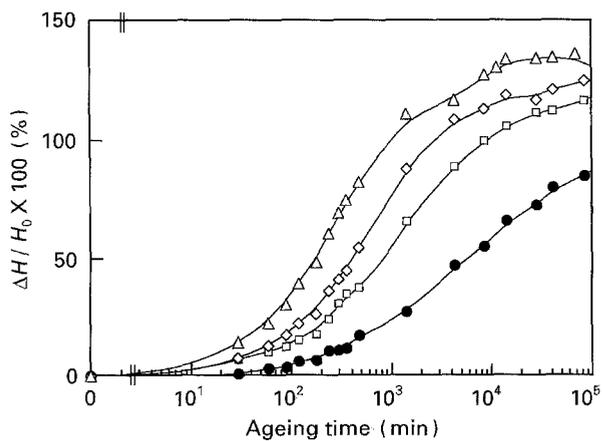
Figure 4 Age-hardening curves of 50AC-G alloys aged at 37 °C: (●) 50AC, (□) 50AC-2G, (◇) 50AC-4G, (Δ) 50AC-6G.
