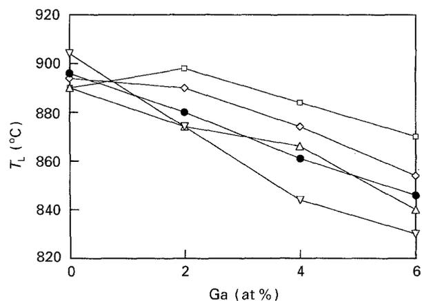
Figure 6 Relation between  $T_L$  and gallium content: (□) 40AC-G, (◇) 45AC-G, (●) 50AC-G, (Δ) 55AC-G, (▽) 60AC-G.
