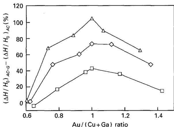
Figure 8 Relation between the Au/(Cu + Ga) ratio and the difference in age-hardening rate between Au–Cu binary and Au–Cu–Ga ternary alloys aged at 37°C for 1 d: (□) AC-2G, (◇) AC-4G, (△) AC-6G.
