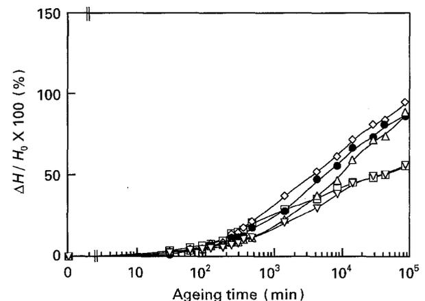
Figure 2 Age-hardening curves of Au–Cu alloys aged at 37 °C: (□) 40AC, (◇) 45AC, (●) 50AC, (△) 55AC, (▽) 60AC.
