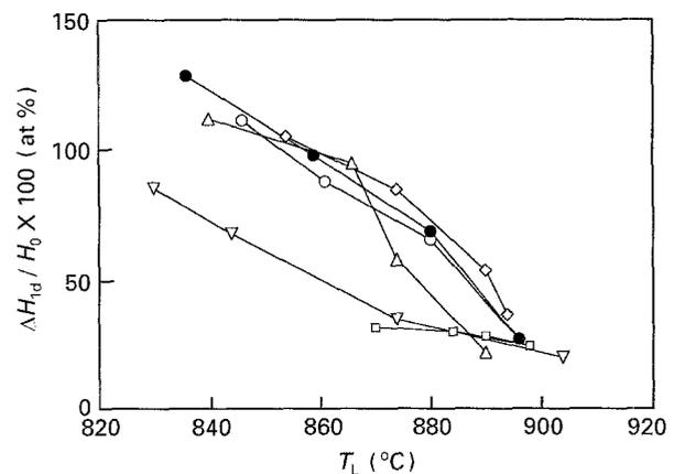
Figure 7 Relation between  $T_L$  and age-hardening rate of specimens aged at 37 °C for 1 d: (□) 40AC-G, (◇) 45AC-G, (○) 50AC-G, (●) 50AC-RepG, (Δ) 55AC-G, (▽) 60AC-G.
